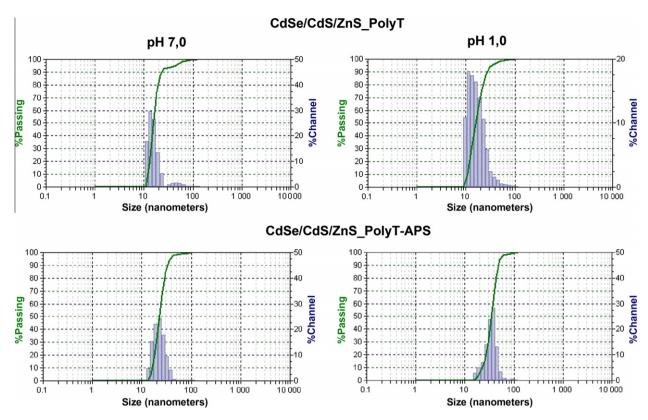
Fig. 2. Hydrodynamic diameter (HD) distribution of QDs PolyT (up) and QDs PolyT-APS (down) at pH 7.0 in deionized water and pH 1.0 in 0.1 M HCl, measured by DLS.
