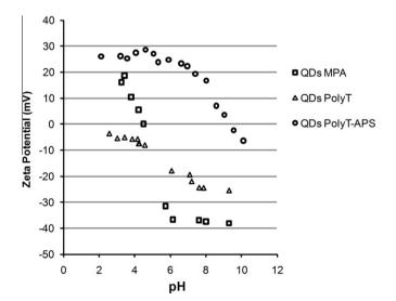
**Fig. 1.** Zeta potential of QDs modified by different functional ligands at various pH values. The measure of zeta potential was performed using a Zetasizer Nano Z instrument (Malvern). pH values of QDs solutions were tuned with 0.01 M HCl (pH 2–10). The concentrations of QDs were 0.1  $\mu$ M.
